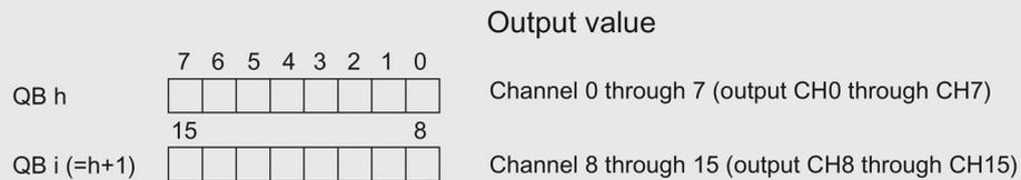
Figure 4-1 Address space for configuration as 32-channel DI 16x24VDC/DQ 16x24VDC/0.5A BA
